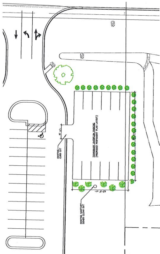
ENLARGED TEMPORARY OVERFLOW PARKING PLAN
