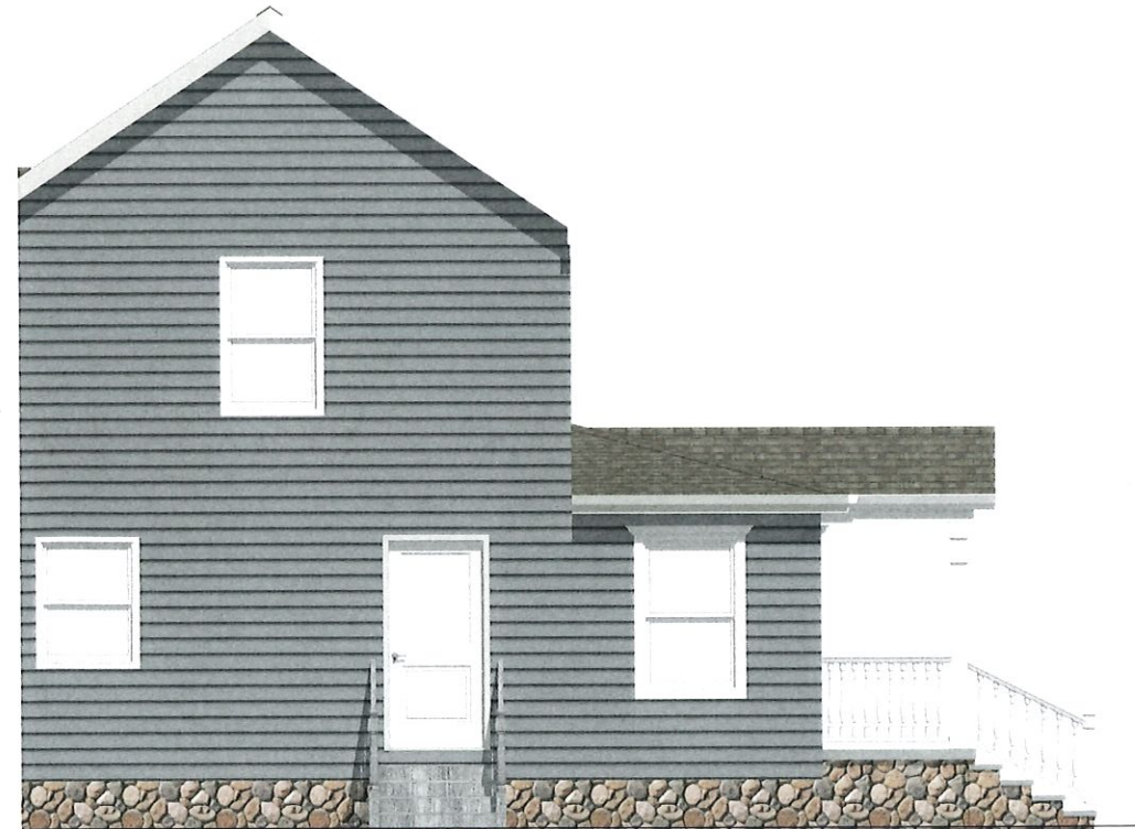
○ NEW PARTIAL SOUTH ELEVATION 1/4" = 1'-0"
